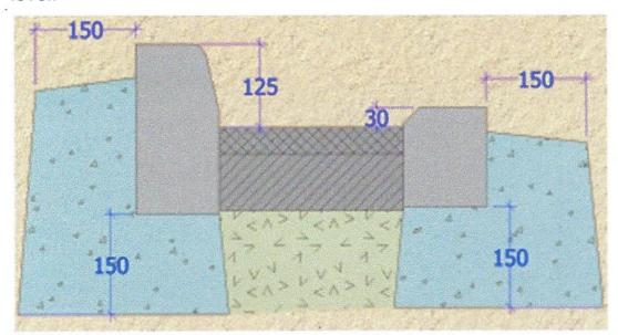
Construction detail for typical kerb
